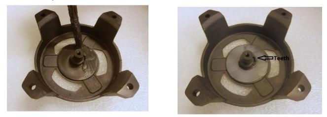
Grease also the upper part of the plastic disk and the central hub of the flash starter, paying attention not to dirty the thread of the hub that you cleaned before.
