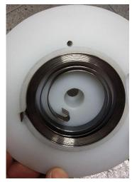
Take a tube of a diameter slightly bigger than the big spring and lean on it the plastic pulley with the big spring downwards. Put a screwdriver in the small hole of 3,5 mm and hit it with a hammer, so that the big spring will fall down in the tube.
