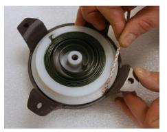
Pre-charge the spring making only one turn of the rope and let it exit from its seat with the help of a hook
