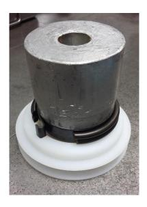
First of all, clean the central thread of the housing with some thinner, to remove any sign of grease from it. Then, grease the bottom of the flash starter and insert the thin plastic disk
