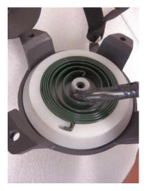
Take the tugger bolt and screw it on the pulley driver, using strong glue on the thread of the screw. Tighten the screw very firmly.
