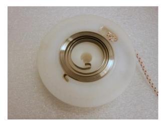
Press in the big spring with the help of a metal cylinder, as in the picture, and a hammer.
