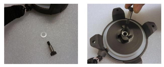
The pulley driver should have some little play. If it hasn't, you can remove the thin washer under the screw. Here you go, the flash starter is ready!
