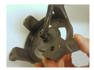
Insert the pulley paying attention to fix the small spring in the teeth of picture 2 of previous page
